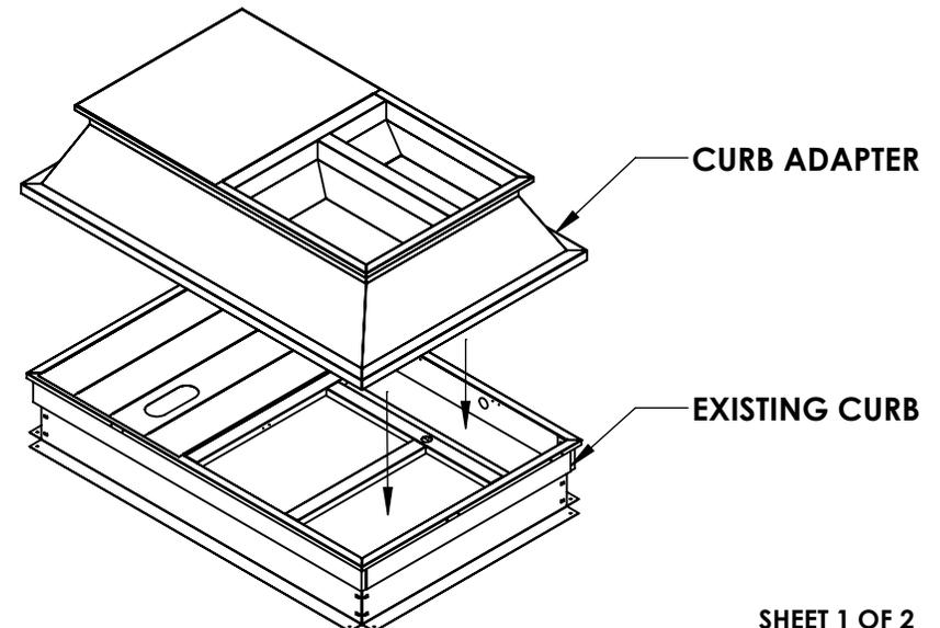
**STEP 4:** IF BLANK OFF PANELS ARE PROVIDED WITH THE ADAPTER, PLACE OVER REMAINING OPENING OF THE EXISTING CURB. FASTEN IN PLACE WITH TEK SCREWS NO MORE THAN 12" APART. ALL SEAMS MUST BE CAULKED WHERE LEAKS MAY OCCUR.
