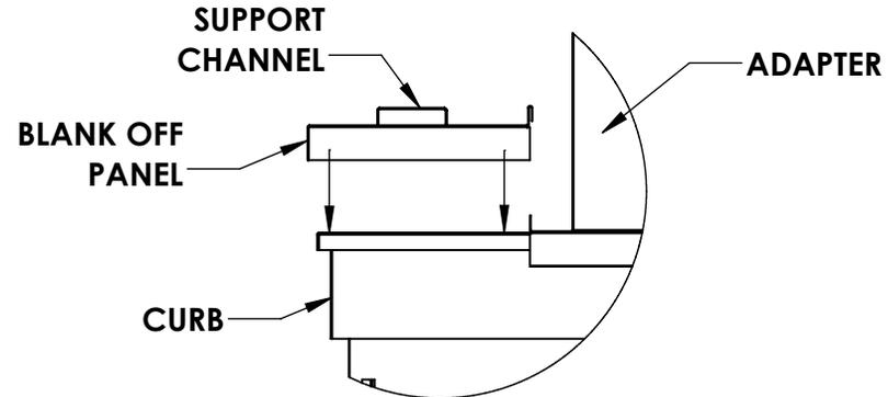
**STEP 5:** IF AN EQUIPMENT SUPPORT IS PROVIDED WITH THE ADAPTER, IT MUST BE PLACED UNDER THE SIDE THAT OVERHANGS THE EXISTING CURB. FIELD SUPPLIED SHIM MAY BE REQUIRED.
