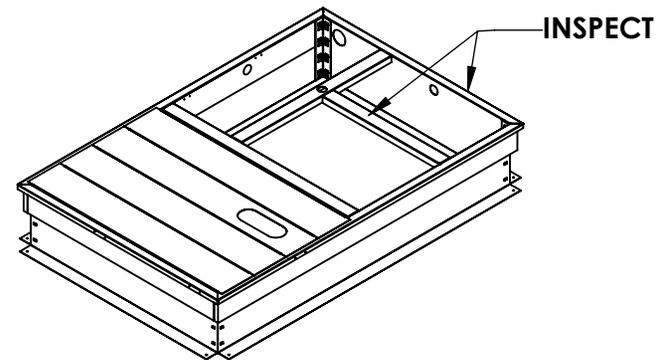
**STEP 3:** SET THE CURB ADAPTER DOWN ONTO EXISTING CURB ALIGNING THE SUPPLY AND RETURN AIR OPENINGS.
