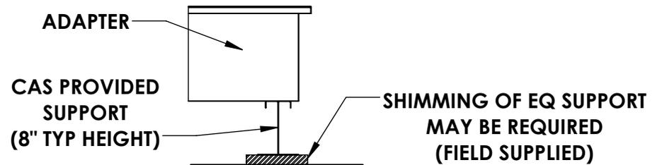
**STEP 6:** APPLY GASKET (PROVIDED WITH ADAPTER) TO THE TOP PERIMETER AND AIR OPENINGS OF THE ADAPTER. CAREFULLY SET THE NEW UNIT DOWN ONTO THE ADAPTER AND CHECK TO MAKE SURE IT IS FULLY SEATED.
